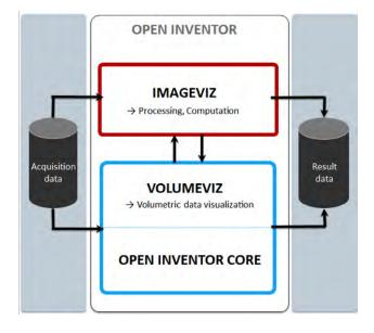
ImageViz is tightly integrated into the Open Inventor SDK and its standard concept of engines, nodes, and fields. Open Inventor data objects can be connected as input to ImageViz processing engines. Moreover, any ImageViz engine's output can be connected to Open Inventor or VolumeViz, allowing easy integration into existing applications.
