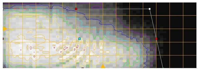
ReflectorCAD® from Breault Research Organization (BRO) is a paradigm-shifting reflector design tool allowing users to make graphical adjustments to the luminous intensity patterns corresponding to individual reflector segments. The program does the rest.
