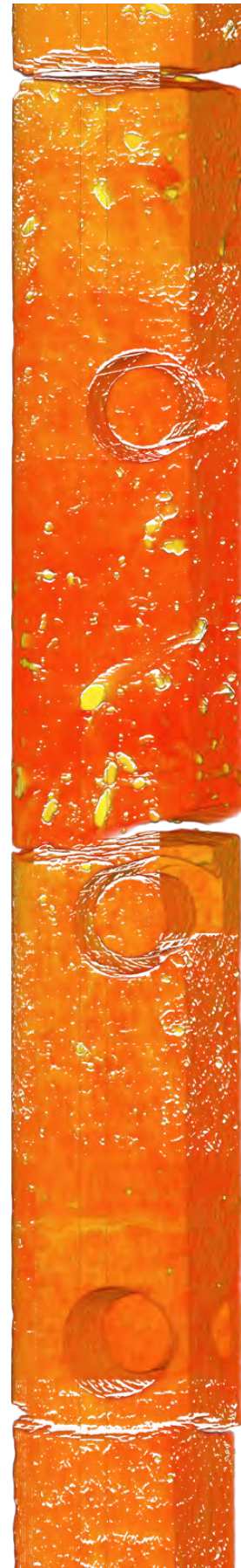
False-color 3D visualization of whole-core CT data. Image detail of five 3-foot segments of whole core aligned and stitched together.
